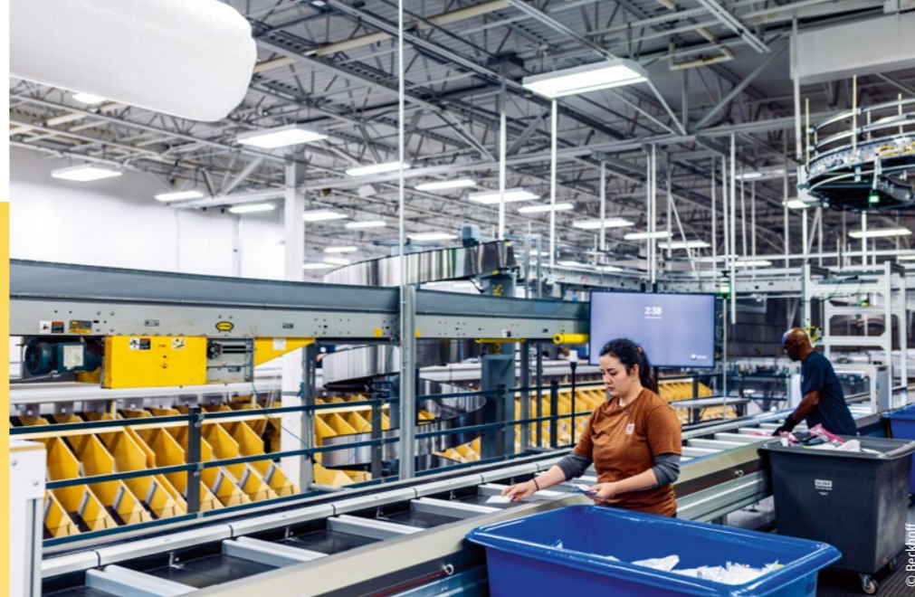
EuroSort's Single Split Tray Sorter, integrates with existing goods-to-person (GTP) systems at Mouser.
