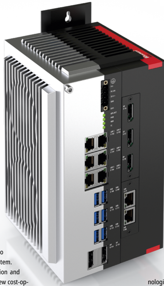
The C6043 Industrial PC with NVIDIA® GPU handles applications with higher demands for 3D graphics or deeply integrated vision and AI program blocks with minimal cycle times.
