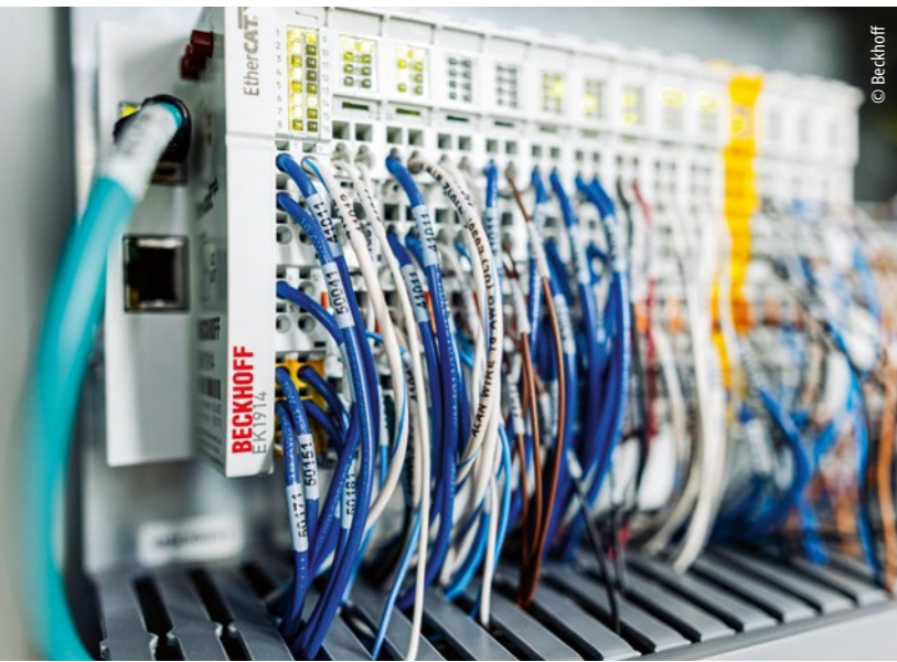
Space-saving EtherCAT Terminals and bus couplers, including the EK1914 coupler with TwinSAFE functionality, combine high-speed real-time communication with functional safety.
