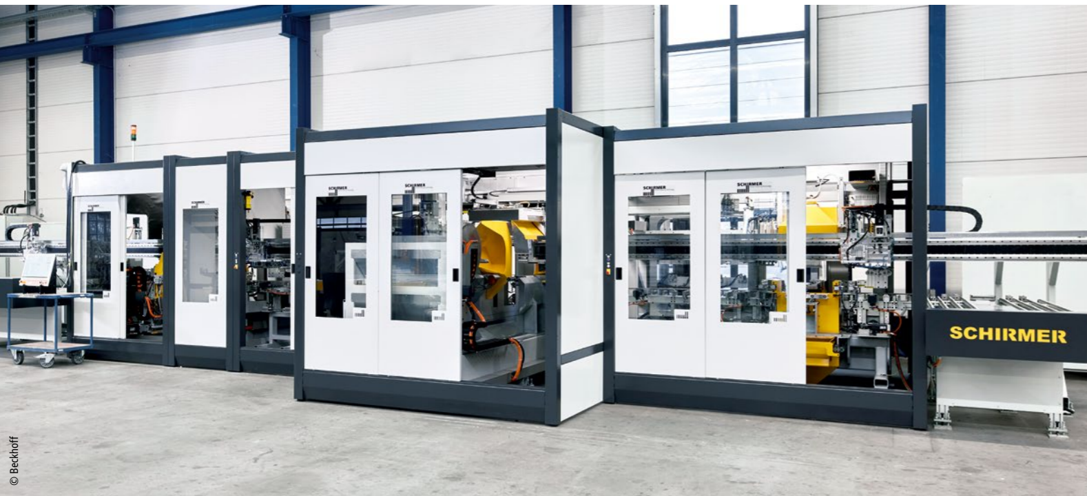
This 14-meter Schirmer machine for the fully automatic processing of PVC window profiles is the first to replace all previously required control cabinets with the MX-System.
