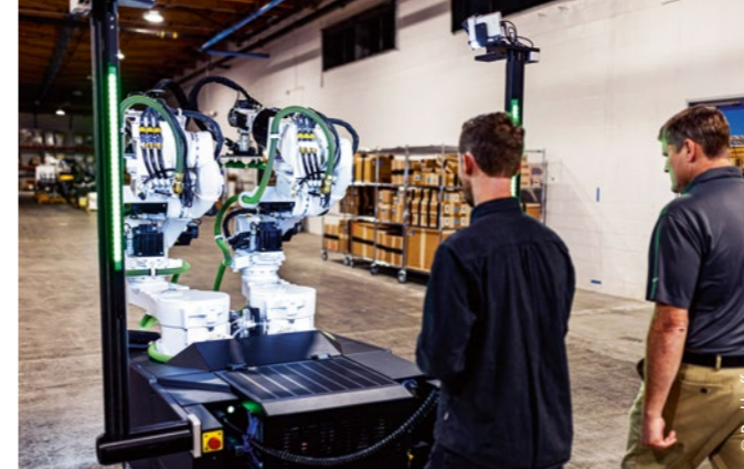
Mech’s ultra-compact rover base moves, spins, and climbs ramps with four steerable wheels.
