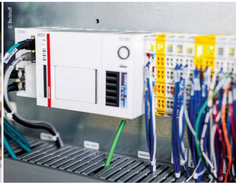
The Beckhoff CX2033 Embedded PC functions as the sole machine controller for the 1400-GEC mailer packaging machine and contributes to boosting scan times.
