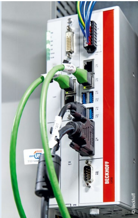
TwinCAT and a C6930 control cabinet Industrial PC handle the path control and coordination of all axes.
