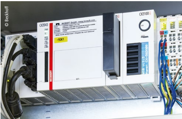
Dynamic synchronization of all axes, safety, HMI, and individual database application – the complete automation project runs on a single CX2043 Embedded PC.
