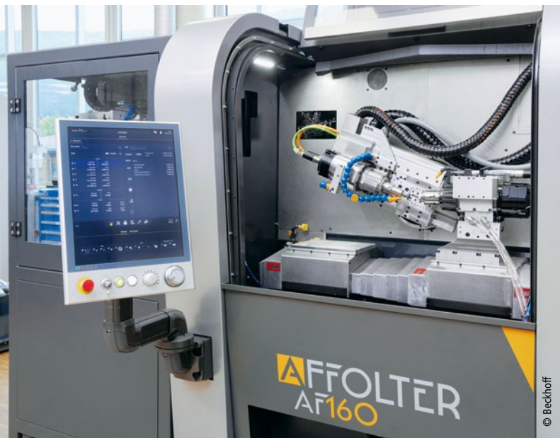
Different CNC machine, same control core: Affolter synchronizes three high-speed spindles with PC-based control from Beckhoff in its own machining centers.
