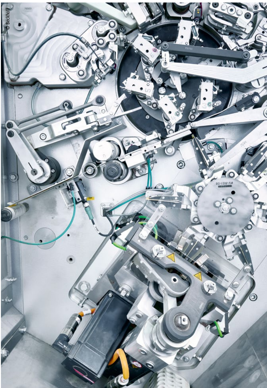
Control of the sophisticated kinematics via TwinCAT NC I and AM8000 servomotors increases the machine cycle as well as flexibility for bag geometry and different packaging materials (e.g., filter paper, wrapping paper, and film).
