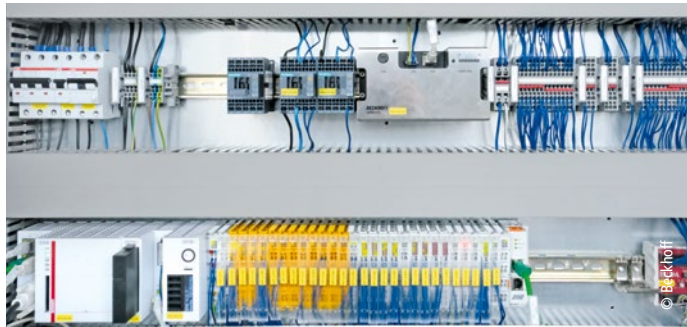
Complete control and monitoring of the prototype runs on a CX2040 Embedded PC (bottom left) with Intel® Core™ i7 CPU and four processor cores.
