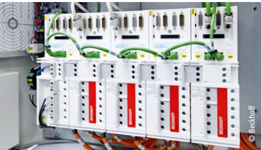
Esco mounts the AX5000 Servo Drives under the machine frame to save space.
