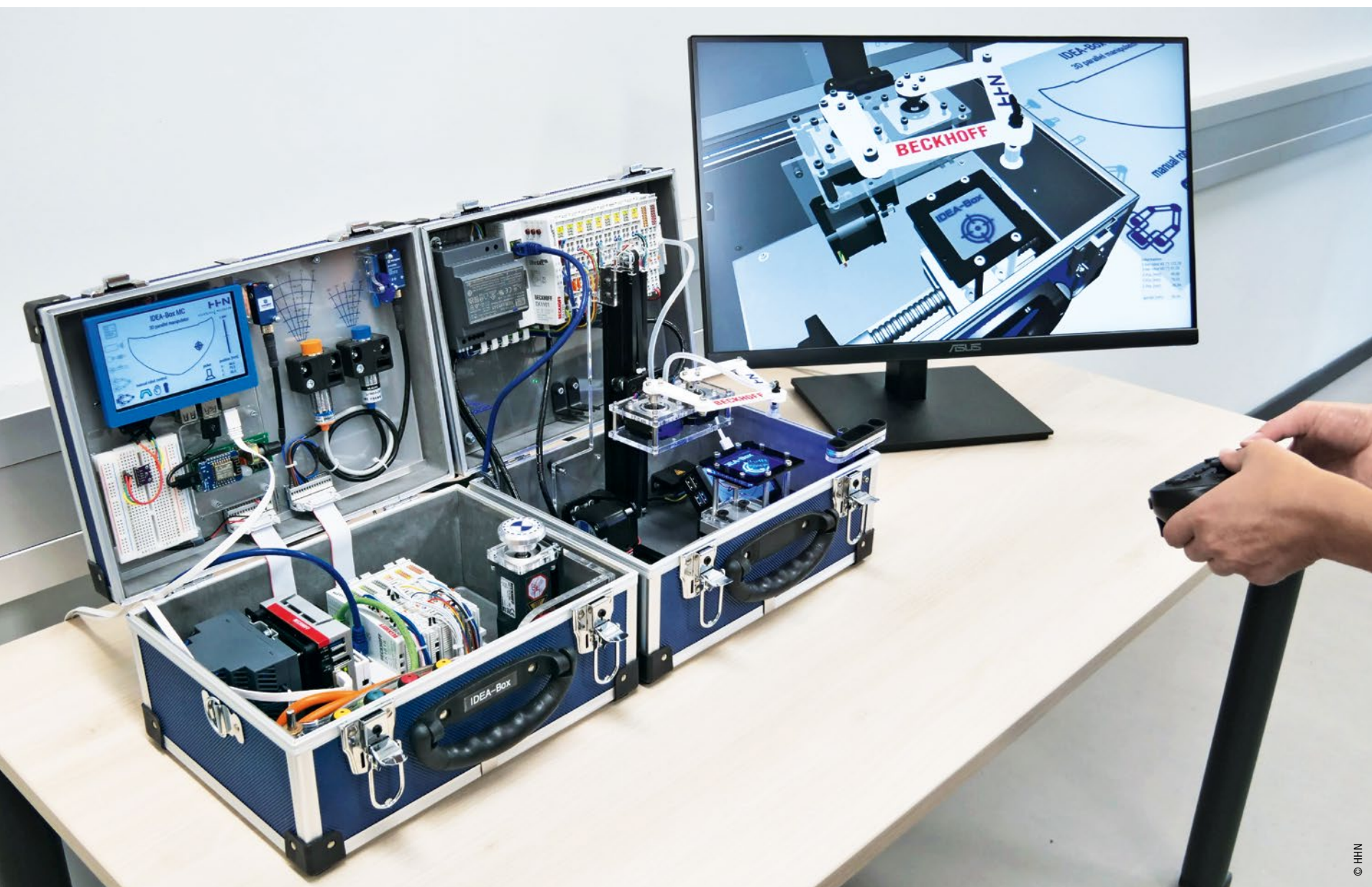
Small and compact cases: The IDEA basic box (left) with the C6015 ultra-compact Industrial PC and the expansion to include more extensive motion functions (right) – where operation via joystick and even hand tracking is possible.
