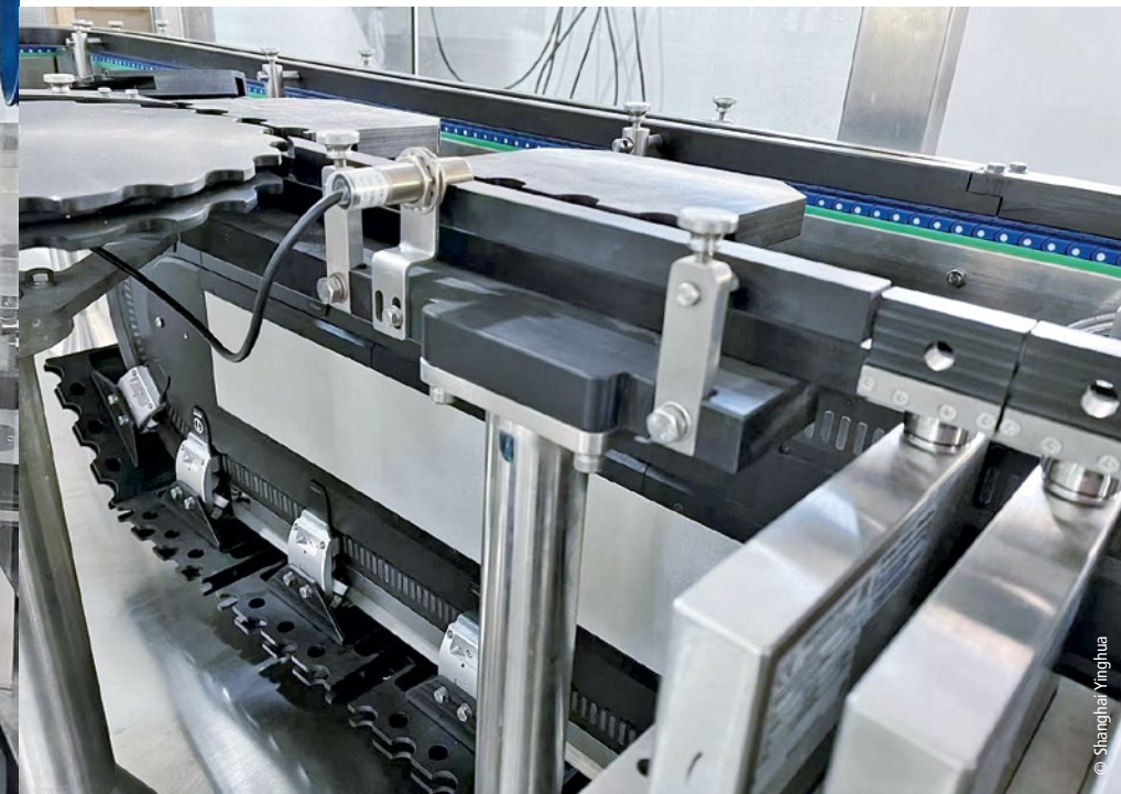
Shanghai Yinghua increases the filling capacity of its pharmaceutical powder systems to 450 vials per minute with the XTS linear transport system.
