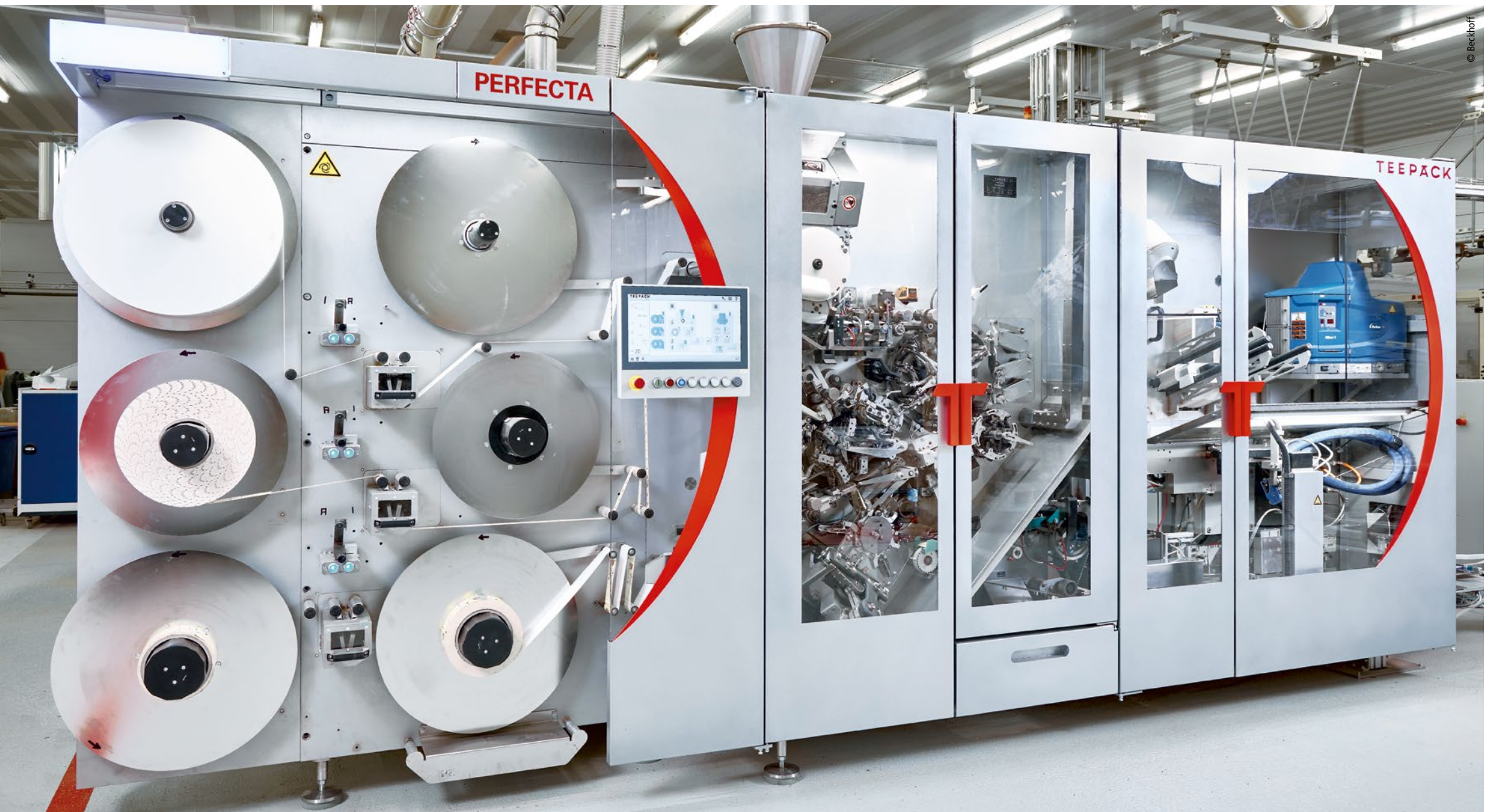
Beckhoff, the system partner: Never before has the tea-bag packaging machine manufacturer Teepack used so many components from a single supplier in a machine as in the Perfecta 450.
