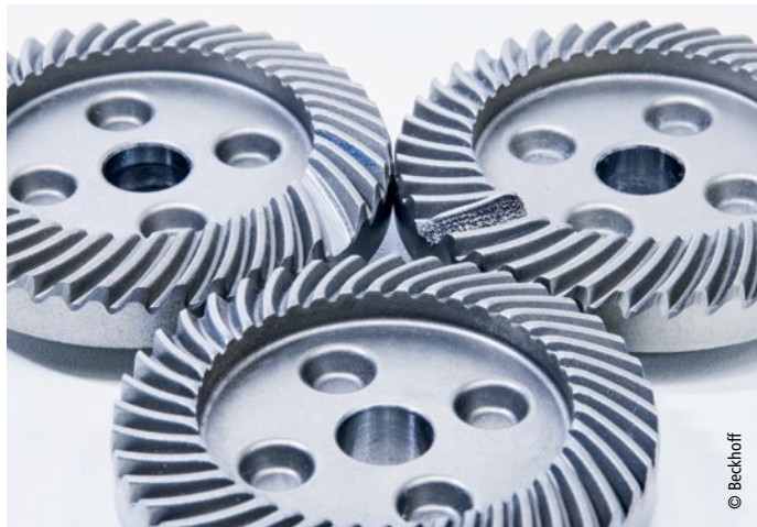
Realistic scenario in circular production: Defective areas of a gear are precisely milled out (left), rebuilt using laser cladding (right), and then finally machined.
