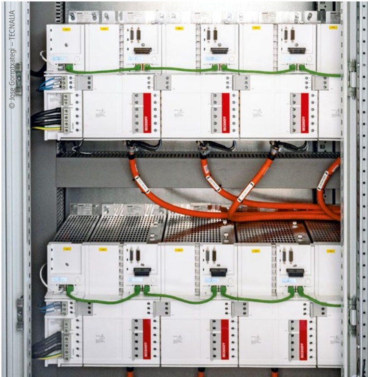
AX5118 servo drives control the eight winch drives of the cable robot and the four axes of the base carrier.
