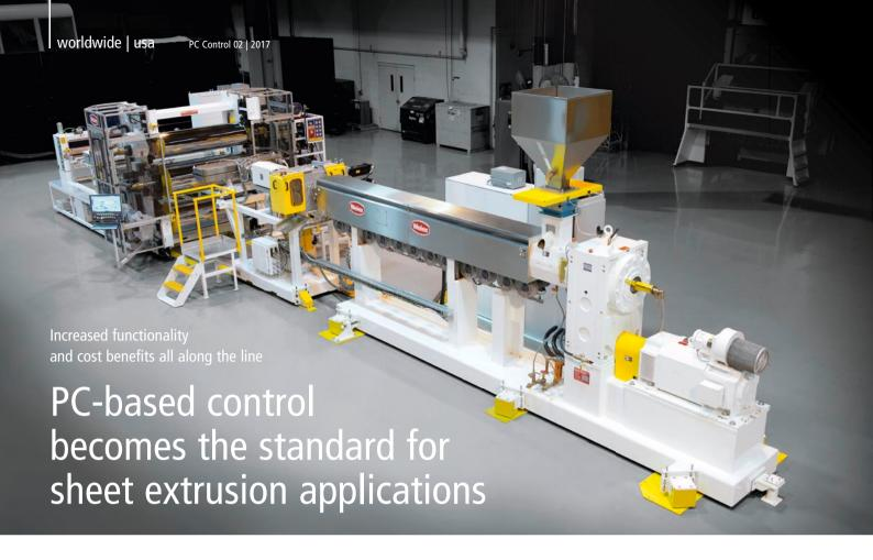
The plastics industry is one of the fastest growing industries in the USA. Many of the plastic products that we use every day start as huge sheets of plastic, manufactured from plastic pellets by sheet extrusion machines. American company Graham Engineering Corporation, based in York, Pennsylvania, manufactures, among other solutions, sheet extrusion machines under the Welex® brand name. These machines rely on Beckhoff controls to optimize their operation and processes.
