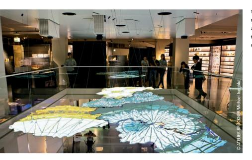
The projection surfaces are suspended on 30 steel cables. Their movement through the three exhibition levels with a height of around 15 meters is individually controlled by servomotors. A total of eight projectors are installed, five of which on the ceiling of the third floor and one each on the other three floors.
